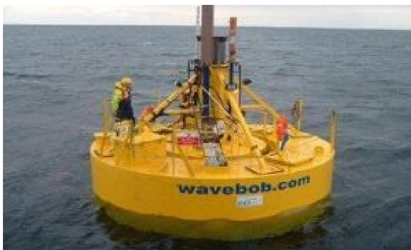
Prototype wave energy device on test in Galway Bay. (Credit: Image courtesy of Marine Institute - Foras na Mara)
